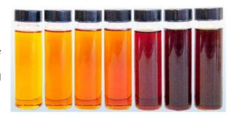
As turbine oil oxidizes, byproducts form and start consuming antioxidant additives, eventually leading to varnish. To achieve longer lubricant life, competitive turbine oils over the past few decades have been formulated with higher and higher levels of base oil refinement and increasing levels of antioxidants. However, this has contributed to varnish and sludge formation in turbine systems.
